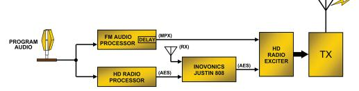
JUSTIN Implementation in HD Radio Air Chain With Dual Audio Processors
